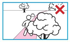
Primary Detection Area (pink) is blocked by obstructions. Reposition the camera so the trees do not obstruct the camera image.
