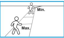
Minimum Detection Size: 1/3 height of image Maximum Detection Size: 1/2 height of image
