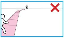
Primary Detection Area (pink) is not the focus of the image. Reposition the camera so the primary Detection Area is the focus of the image.
